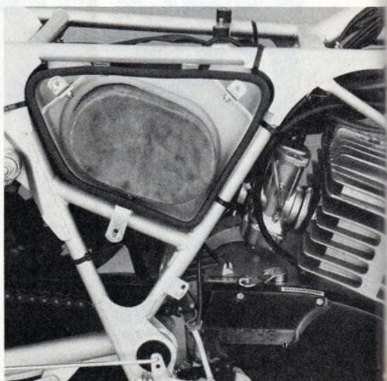
Airbox features water baffles, a drain, Twin Air filter and large volume in front of the carburetor.
