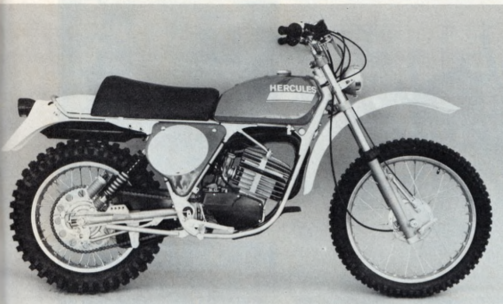
Engine sits high in frame out of harm's way. A tough plastic skid plate adds protection and deflects mud.
