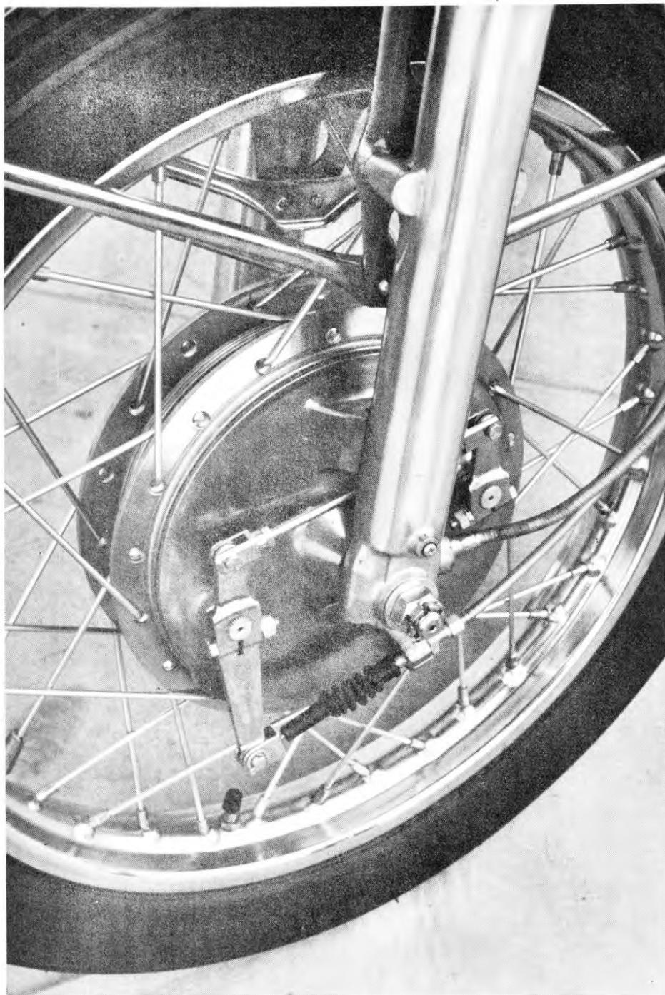
**Although the front brake worked, we felt it would be better to have more stopping power. It's the double leading shoe type.**
