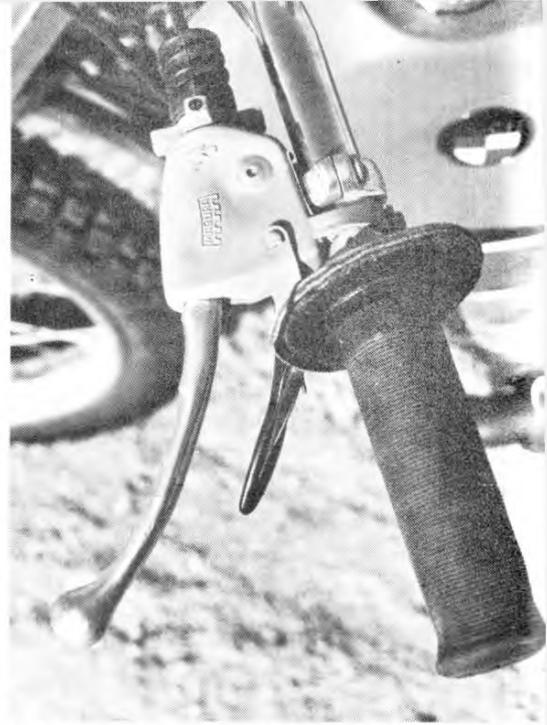
**Fully enclosed and adjustable Magura levers are standard. Hand grips and compression release are accessory components.**
