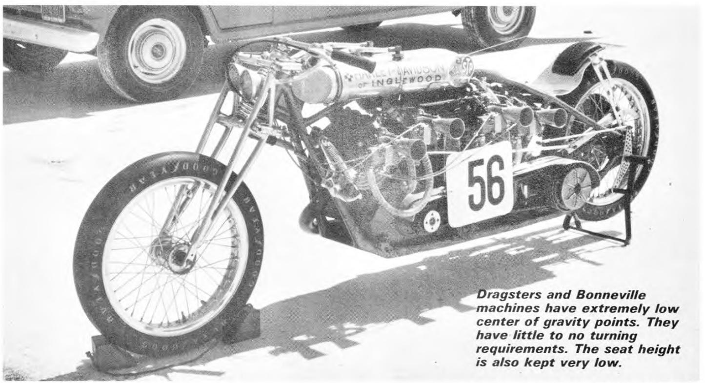
***Dragsters and Bonneville machines have extremely low center of gravity points. They have little to no turning requirements. The seat height is also kept very low.***
