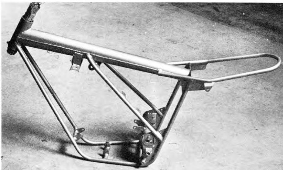
***In an attempt to acquire maximum strength and minimum weight, the AJS motocross frame uses a combination double cradle and semi-backbone construction.***
