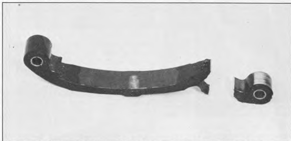
Slipper for the timing chain tensioner broke just below its pivot. Lots of noise, no damage and an expensive repair.
