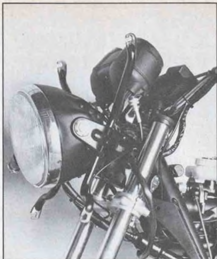
Normal BMW halogen headlight is mounted to fairing brackets. A rubber boot mounts between the fairing and the headlight.
