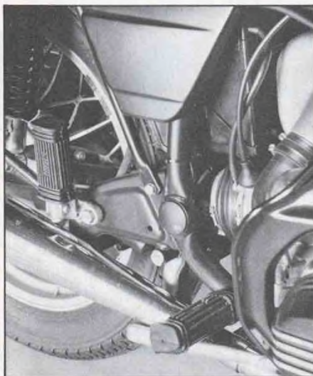
Passenger footpegs as well as rider pegs are adjustable, allowing a more comfortable seating position. Adjustment is limited, however, and the distance from fairing edge to front of saddlebags makes for a tight fit with a passenger aboard.
