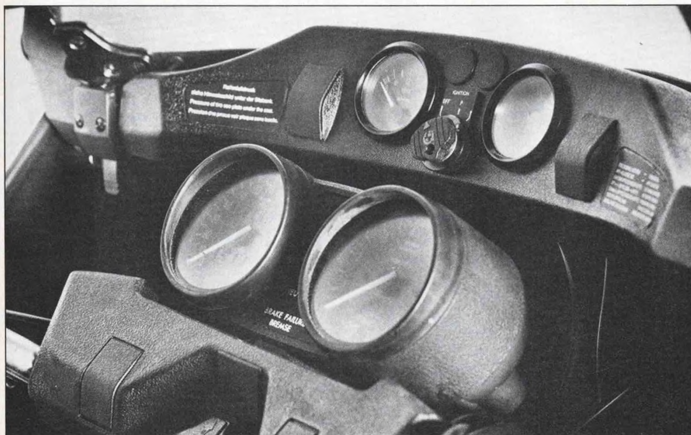
RT fairing has a dashboard for voltmeter, quartz clock, ignition switch, and has room for additional switches. RT uses the same gauges as last year's BMWs, rather than the larger gauges from the R65.
