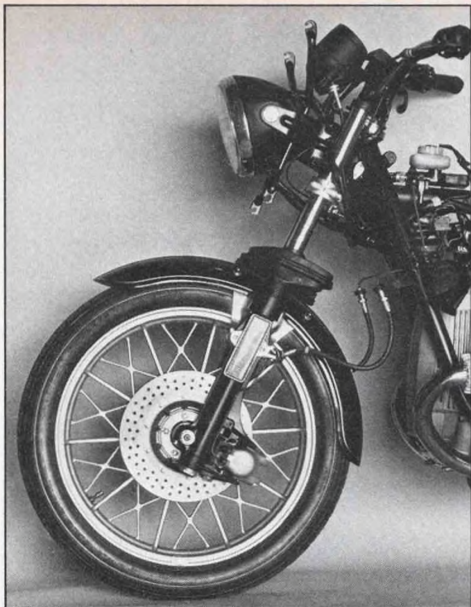
Long-travel front forks have 7.9 in. of travel. Dual front disc brakes are drilled, require heavy lever pressure for normal stops, but work well in the wet.
