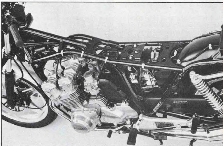
CB750F frame is gusseted in the steering head area, built with double-wall tubing at stress points and has downtubes with greater wall thickness than used in similar K model frame.
