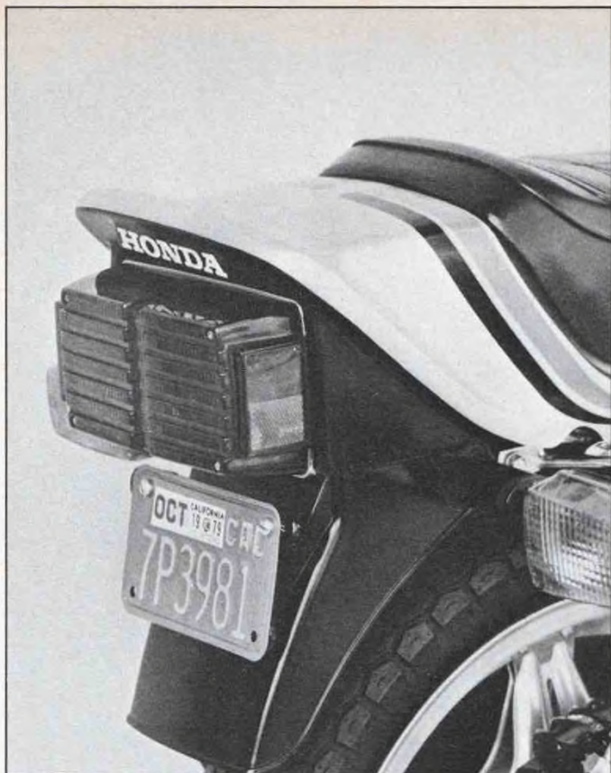
Taillight is the same as used on the CBX, has two bulbs and is very bright.
