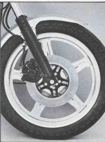
Front brakes are strong, but developed pulse and squeal within 100 miles of hard test use.
