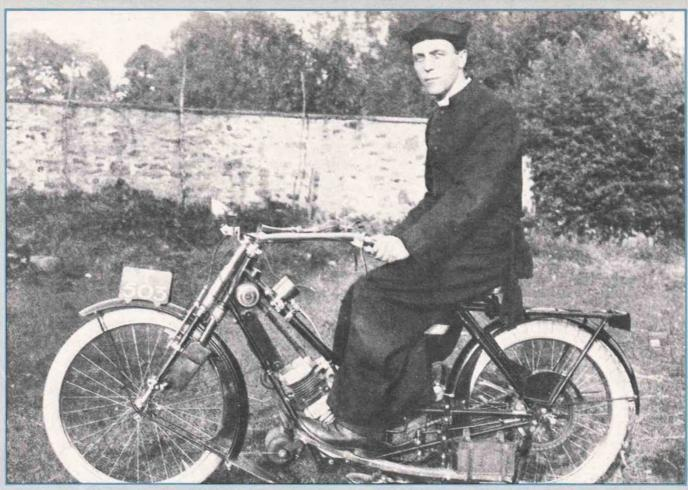
loaded up, and by the time Scott got into proper production with a 450cc engine, he had gone to water cooling with a proper radiator on the front down-tube. Even at this time, undoubtedly influenced by steam-engine practice, the machine was fitted with horrid little drip-feeds which doled out oil to the mains and rods. No petroil for Alfred Scott.
