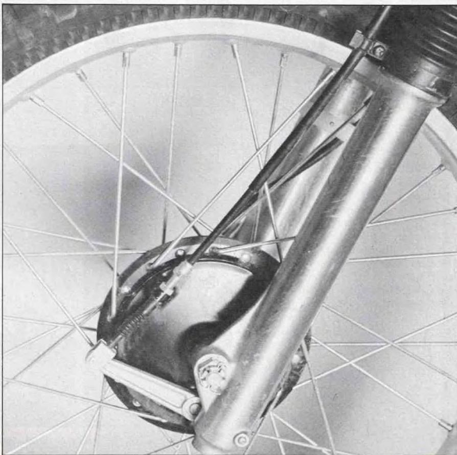
Leading axle forks offer average travel, handle large bumps better than small ones.
