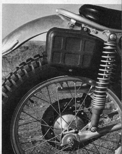
mounting point. Use of a longer swinging arm is thus allowed, weight is saved, and available space between the carburetor and rear fender is increased.
