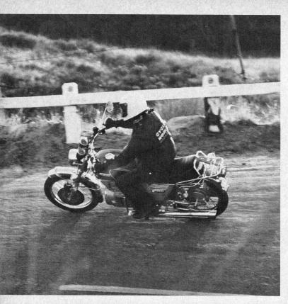
front works well as long as the front brake lever does not bottom against part of the throttle housing (ours did when we took delivery). The rear drum unit is equal to the front in feel and stopping ability.
