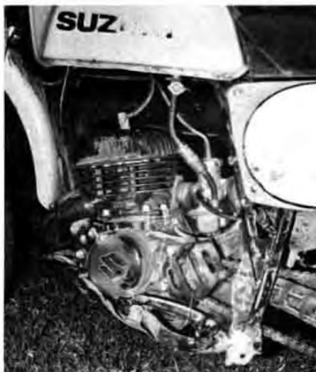
Yes, it was a tough test; witness the worn-away letters, the missing sidestand and the safety wire looped around the gear lever just in case it worked loose again. The engine was still running strong at the finish and the post-test teardown showed minimum wear.
