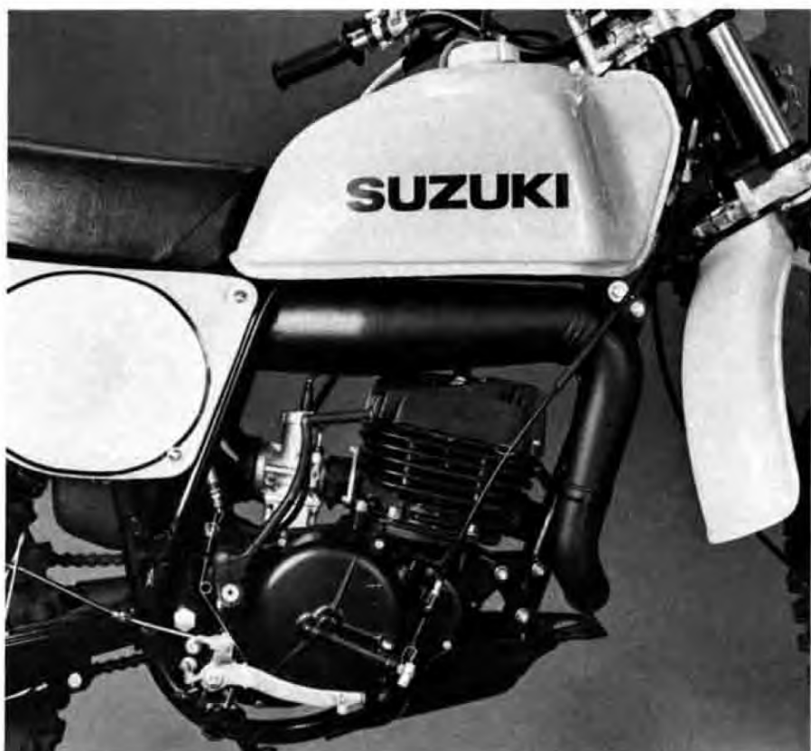
The PE250 motor is best described as a new engine, with different bore, stroke, displacement and timing, inside RM250 cases.
