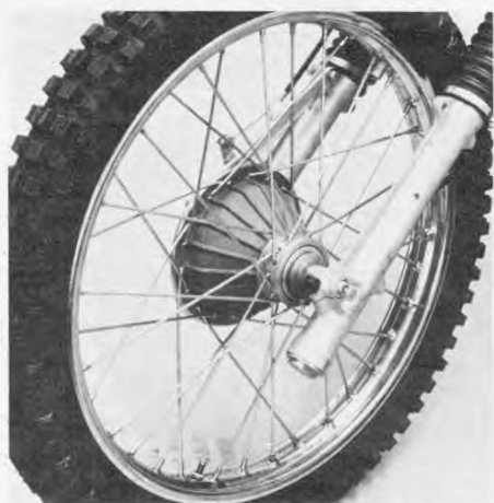
All the nine gauge spokes stayed tight. Front wheel is light. Fork action is the best.
