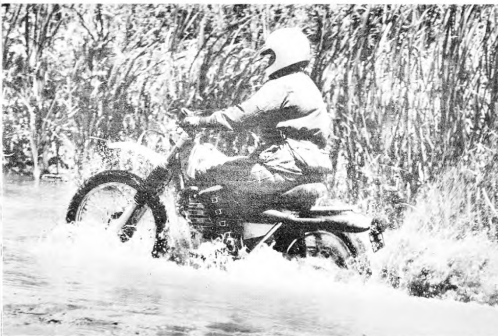
After drowning bike like this for an hour the Twin-Air filter passed water. Ignition never faltered.
