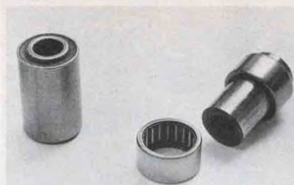
Rubberized swing arm bushings have been replaced with needle bearings, which eliminate flexing.
