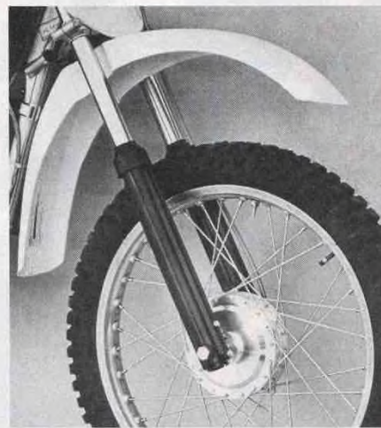
The late version Husky fork delivers supple ride with new damping system and 8 1/4-inches travel.
