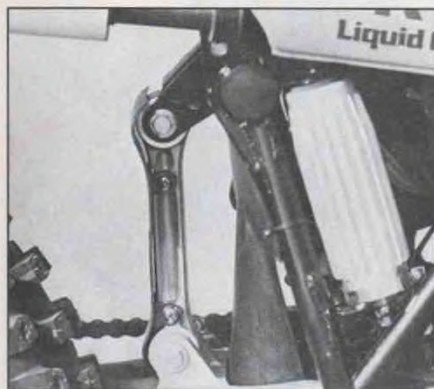
The 1983 Uni-Trak features the same working parts as the KX500. A vast improvement in rear wheel action and a loss of three pounds is the net gain.
