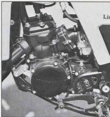
Larger ports are the main feature on the new KX engine, although external appearance hasn't changed since '82. More ponies makes the KX easier to ride.
