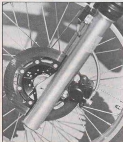
Front brake caliper is bigger, brake action is stronger. Locking up the front wheel is no problem at all.
