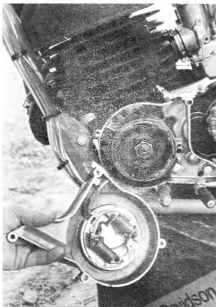
By just removing the cover you will have the whole primary ignition unit in your hand. The backing plate is permanently located in the cover, timing adjustments are done by moving the pick-up, seen at the outside of the flywheel at five o'clock, right in front of the folding shift lever.
