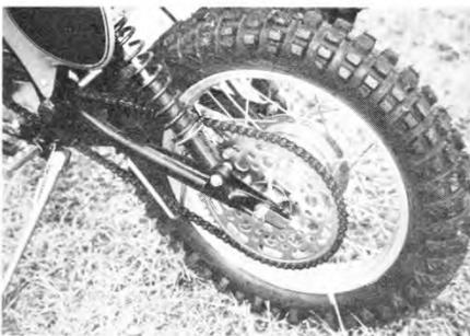
Simple but very sturdy chain guide keeps the chain on the Rococo-sprocket.
