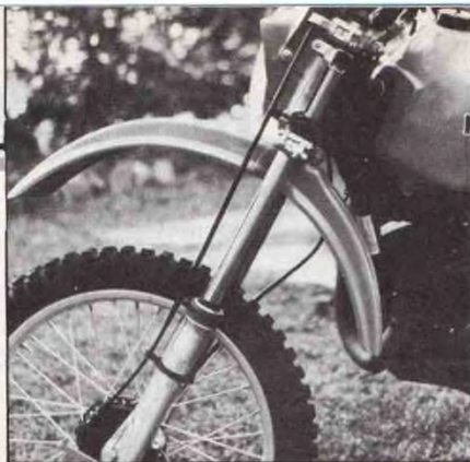
For the best, safest operation, the front brake cable should run a straight line right up to the lever.
