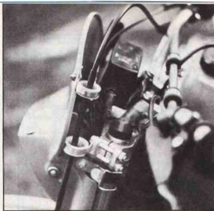
You may find it's necessary to add another loop to the top of the front brake cable. On this bike, the extra loop keeps the cable away from the enduro clock.
