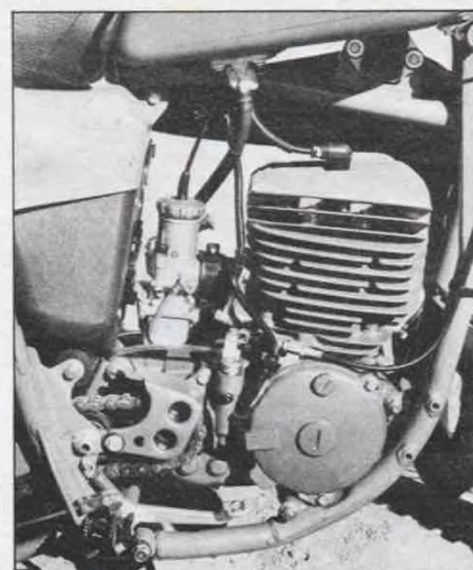
New cylinder was built to fit double-tube frame, porting and lower end are essentially the same as last year.
