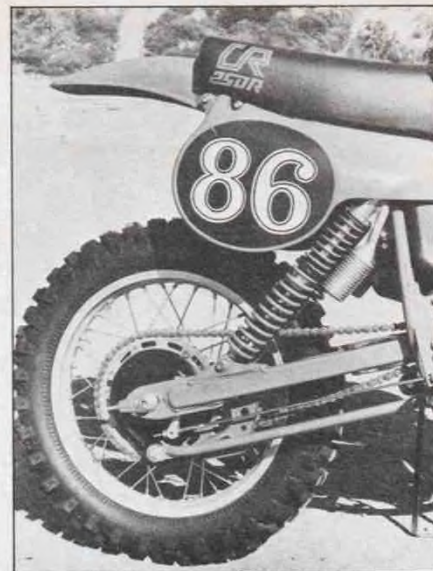
Big news for this year is new rear shocks. Units are adjustable, need better springs.
