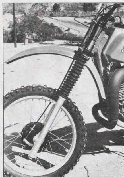
'80 forks feature air caps, better damping than '79. They work very well.
