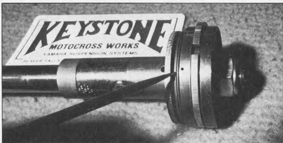
**Here's what the new damping unit looks like fully rebuilt.**
