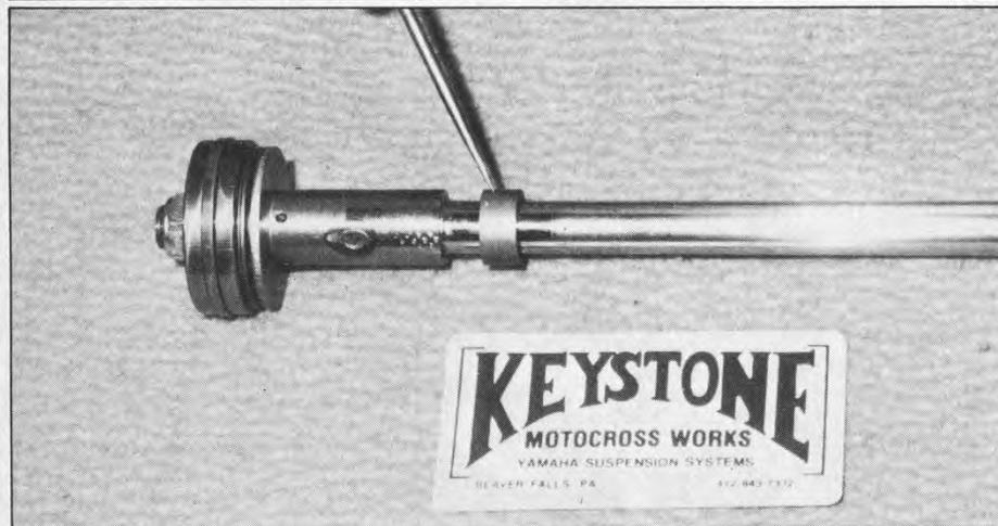
*For the Keystone Travel mods, the large stock spacer on the damping rod is replaced with a smaller one.*
