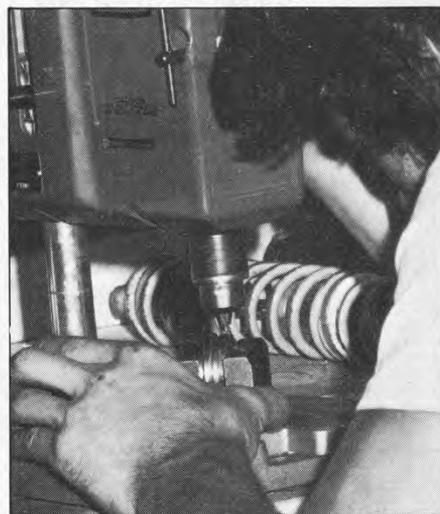
*For better rebound damping, the damping piston is drilled out to relieve back pressure.*
