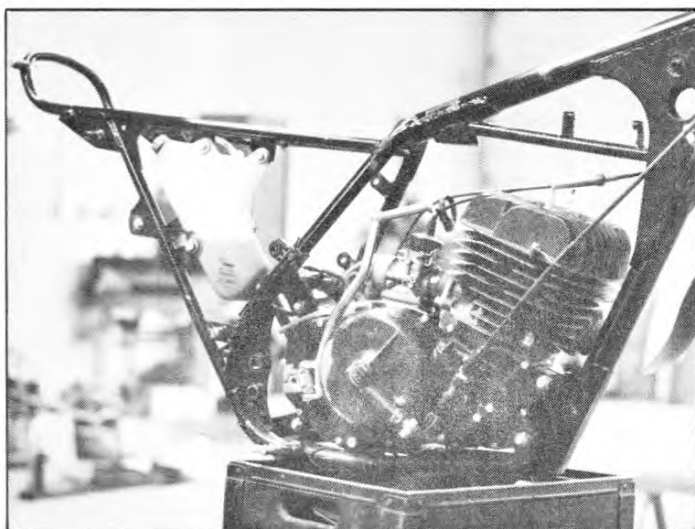
2 The Suzy is stripped almost naked, removing the gas tank, seat, coil, ignition box, air box, rear swing arm assembly, rear fender and exhaust pipe.
