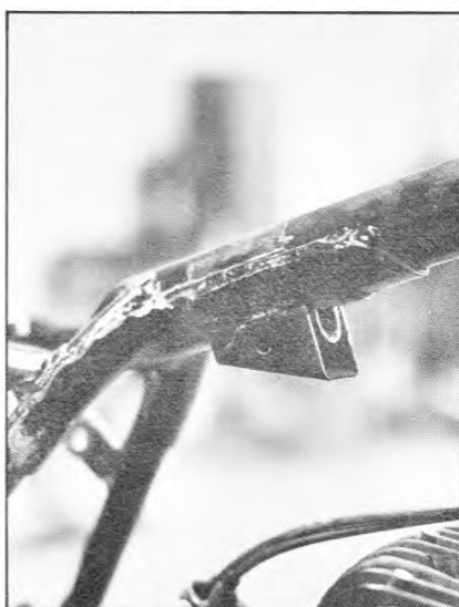
5 The bracket is cut flush with the flange to enable the new head brace to fit tight.
