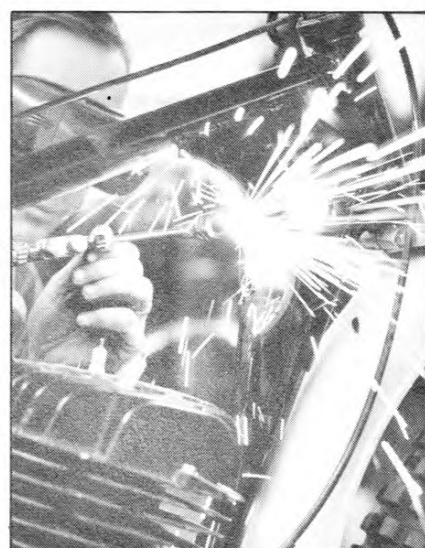
6 A radius is cut in the big front frame gusset to allow the shock to pivot once it's in place.
