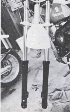
Slide the tubes into the triple clamps, and tighten the bottom two pinch bolts. Raise the tubes 11/2" above the top clamp before completely tightening.
