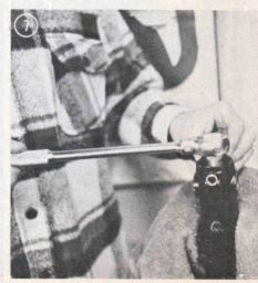
steady basis have a center stand, or orange crate; that'll do fine. Remove the front wheel and drain the fork oil. Loosen the top pinch bolts and remove the stanchion caps. Loosen the other pinch bolts and remove the springs; you're ready to start on the dampers. This is where you need the tool. For the damper bolt, an 8mm Allen is needed. We found that an impact works good for this job. It seems to shock the bolt loose quicker than turning with a ratchet.
