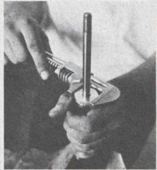
Loosen large cap on body of shock. A large crescent will do an adequate job, but the right size wrench is better. We had nothing that would fit-hence the cruder tool.
