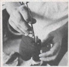
Slip oil retaining sleeved cup over compressed shaft. Do this gently to keep oil from surging out. Make sure oil retaining sleeve is centered over inner body.
