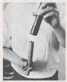
When re-installing inner body, make sure washer placement is centered.
