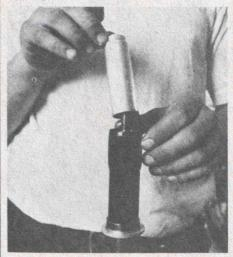
Remove oil retaining sleeved cup from body and slide upward over depressed
