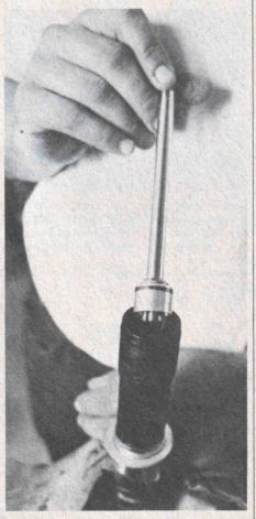
Install piston shaft assembly. By gently using small screwdriver, piston ring can be compressed to allow unit to slip in.
