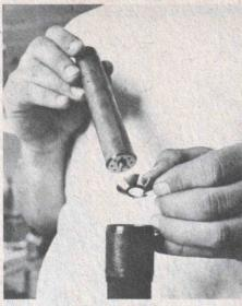
Pull out inner body (sleeve) and drain. Clean all parts thoroughly and check for wear.
