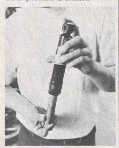
Hold inner body upside down and slowly slide housing over it, making sure that locating washer is not disturbed.
